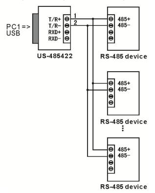
3. Half duplex connection between GM-485422 interface converters
