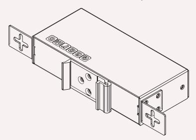
Insert the top of the DIN Rail Clip onto the DIN Rail Track, then gently push the bottom of the hub to secure it to the DIN Rail Track.
