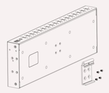
Insert the top of the DIN Rail Clip onto the DIN Rail Track, then gently push the bottom of the hub to secure it to the DIN Rail Track.
